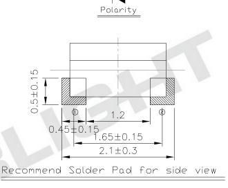
Suggested pad dimension is just for reference only. Please modify the pad dimension based on individual need. Note: Tolerances unless mentioned ±0.1mm. Unit = mm
